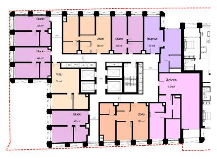
Image 8: potential C3 Use Class conversion of Tower A floorplate
